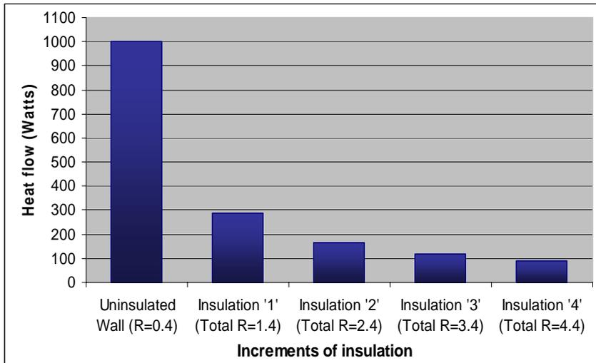
**Figure 1. Diminishing returns effects from adding increments of wall insulation<sup>2</sup>**
